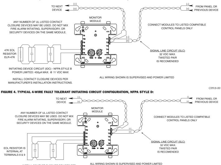
INSTALL CONTACT CLOSURE DEVICES PER MANUFACTURER'S INSTALLATION INSTRUCTIONS.
